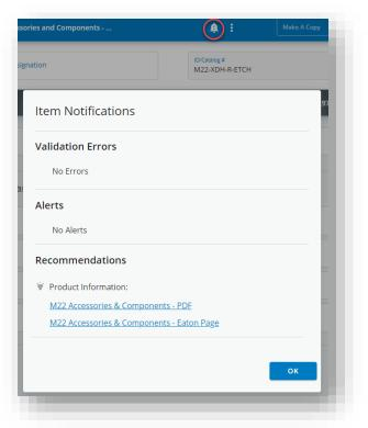
When you click **Bell icon** or when you save your configuration, the system will check for Validation Errors and Alerts and will display the Technical Data Sheet for M22 Accessories and Components.
